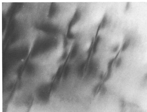
Figure 8 Clusters of niobium atoms in the structure of Fe–3.5 wt % Nb alloy aged for 7 h at 600 °C ( \times 150\,000 with foil normal to [001] ).
