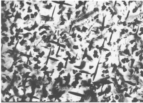
Figure 5 \text{Fe}_2\text{Mo} particles in the structure of Fe-15 wt % Mo alloy aged for 20 h at 550 °C ( \times 32000 with foil normal to [001] ).
